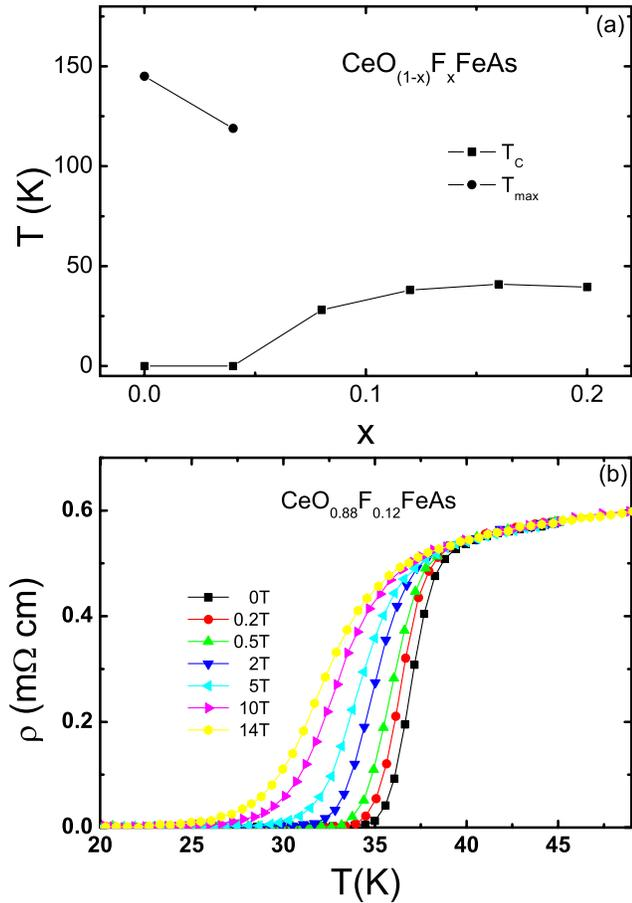
FIG. 3 (color online). (a) The phase diagram showing the anomaly (circle) and superconducting transition (square) temperatures as a function of  $F$  content. (b) The resistivity vs temperature curves under selected magnetic fields.
