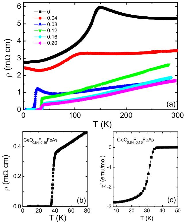
FIG. 2 (color online). (a) The electrical resistivity vs temperature for a series of  $\text{CeO}_{1-x}\text{F}_x\text{FeAs}$ . (b)  $T$ -dependent resistivity in an expanded region for  $x = 0.16$  sample. The superconducting transition with sharp onset temperature at 41 K is seen. (c) Real part of  $T$ -dependent ac magnetic susceptibility.
