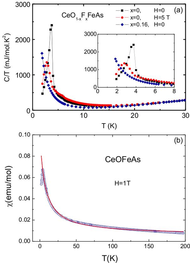
FIG. 5 (color online). (a) The plot of  $C/T$  vs  $T$  for the pure CeOFeAs sample at  $H = 0$  and 5 T, and the  $\text{CeO}_{0.84}\text{F}_{0.16}\text{FeAs}$  sample at  $H = 0$ , respectively. The inset shows the plot in an expanded low temperature range. (b) The  $T$ -dependent magnetic susceptibility of pure CeOFeAs sample. The red (or gray) curve is a fit to the Curie-Weiss law. The sharp drop below 4 K is due to AFM ordering.
