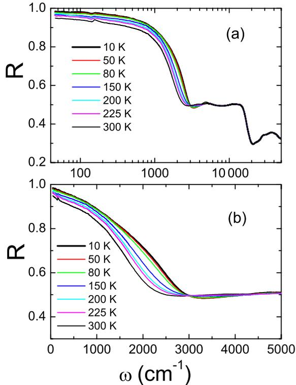
FIG. 1 (color online). (a) The  $T$ -dependent  $R(\omega)$  in the frequency range from 50 to 50 000  $\text{cm}^{-1}$  on a logarithmic scale. (b) The expanded plot of  $R(\omega)$  from 50 to 50 000  $\text{cm}^{-1}$ .
